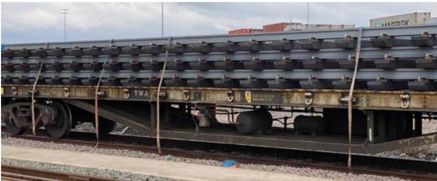
Prefabricated Sicut Plastic Composite Sleeper track panels ready for delivery to site
